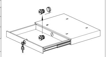
STEP 1:Open the drawer, remove the USB extension(5V3.1A), and unscrew the plastic nut
