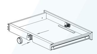
STEP 2: Insert the USB extension (5V3.1A) into the hole at the back of the drawer and secure it with a plastic nut
